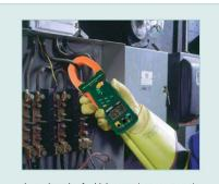
Large jaw size for high current measurements
